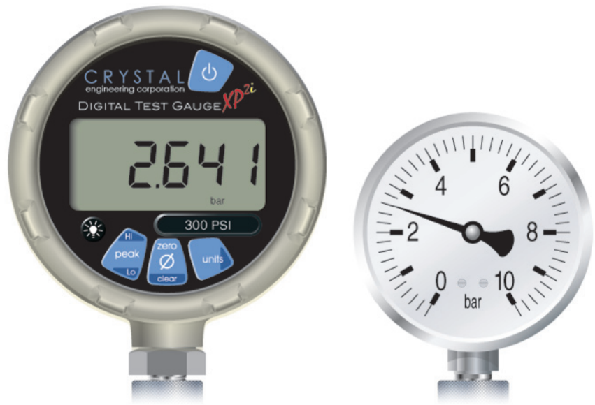
Figure 4. Checking the accuracy of an analog pressure gauge against the display of the XP2i digital pressure gauge.
