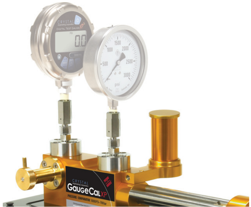
Figure 3. The GaugeCal XP Pressure Comparator can be configured with an XP2i digital test gauge and a gauge to be tested, in either of the two ports. The above example also has the optional Fine Adjust option installed.
